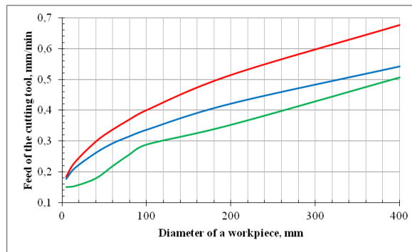
Figure 1 – The dependencies of feed of the turning cutters from the workpiece diameter: — the round carbide insert (mechanically clamped), — the rhombic carbide insert (mechanically clamped), — the triangular carbide insert (mechanically clamped).
