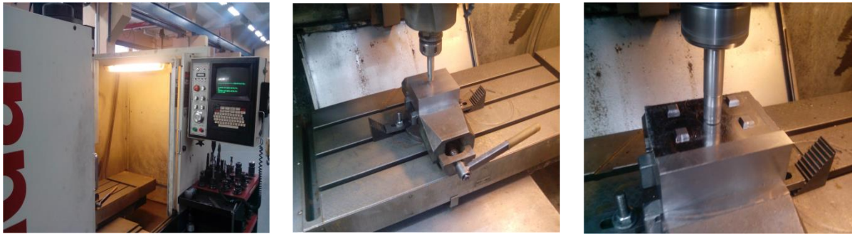
Figure 6 – The CNC milling operation.
