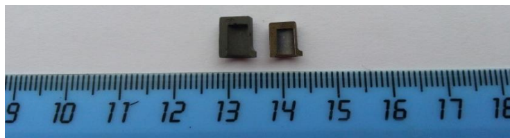
Figure 2 – The castings before heat treatment (left) and after heat treatment (right).
