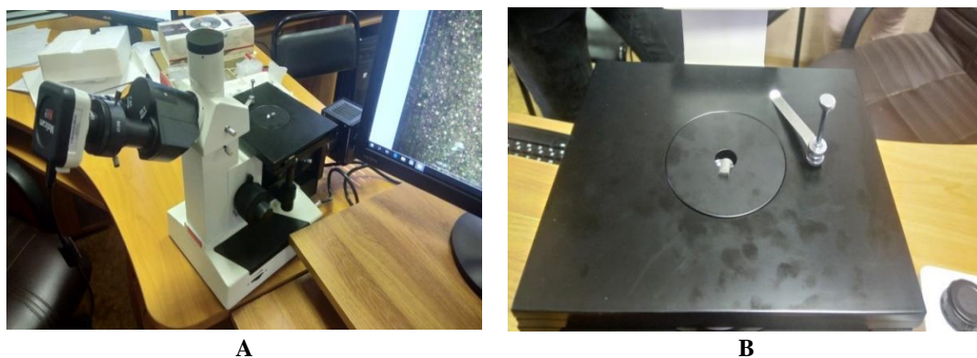
Figure 3 – The equipment for realization of the research: A – general view of the metallographic microscope; B – the microscope stage with the installed casting.
