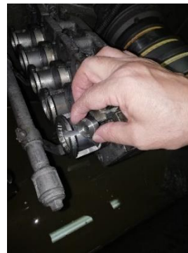
Figure 5 – The die for installation in the seats of the drawing machine of Italian production.
