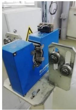
Figure 7 – The laser device for measuring of the diameter and the oval of wire.
