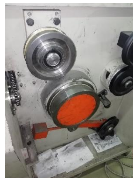
Figure 6 – The guide and bypass mechanisms: A – the drawing machine of Chinese production; B – the drawing machine of Italian production.
