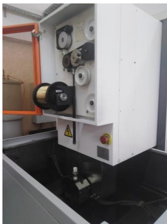
Figure 1 – The general view and the technical characteristics of the CUT 20 (GF AgieCharmilles) electrical discharge machine.
