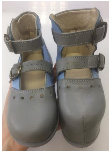
Figure 20 The design of shoes with a seam on the vamp
