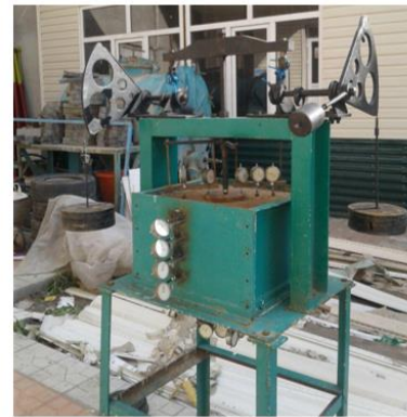
Fig-2. Bench scheme of indicators for measuring displacements, general view of the bench of measuring equipment: 1-volume tray with dimensions A \times B \times H = 45 \times 45 \times 30 \text{ cm}^3 ; 2-lower plate of the pressiometer; 3-upper plate of the pressiometer; 4-tared finely grained sand; 5 - coarse sand; 6-masses; h_I -V-horizontally directed indicators.
