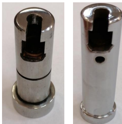
Figure 3 – The upper (left) and lower (right) devices for tensile testing of the round specimens.
