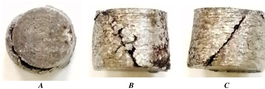
Figure 6 – The fractured round specimen after compression: A – fracture of material (the view from the end surface); B and C – cracks along the diameter.
