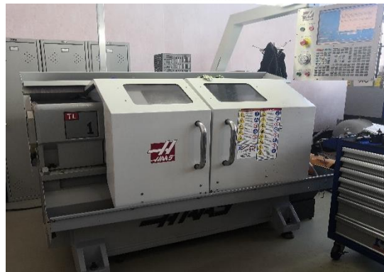
Figure 1 – The structure of the "Haas TL-1" CNC lathe machine.
