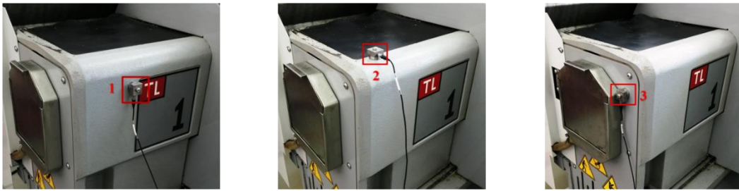
Figure 2 – Locations of the sensor on the casing of the spindle assembly for vibration measurement.
