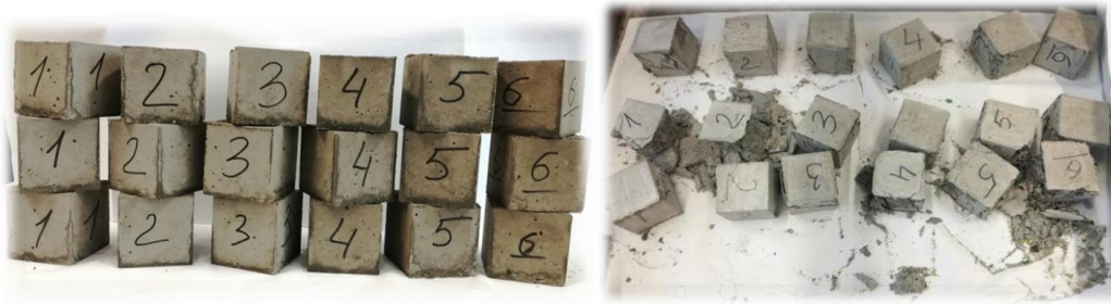
Figure 2. Appearance of concrete specimens before and after testing compressive strength tests
