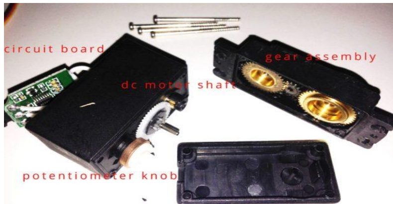
Figure 2. Servo motor structure
