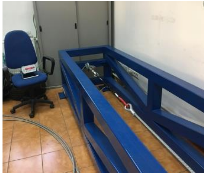
Figure 3 – Static resistance test stand
