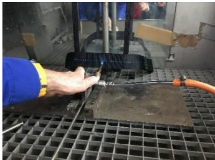
Figure 1 - Flame exposure system
