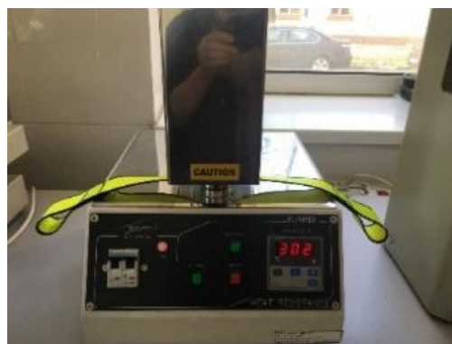
Figure 2 - Apparatus for testing the contact heat resistance
