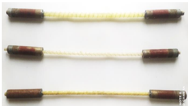
Figure 1. Samples of fittings prepared for elongation testing
