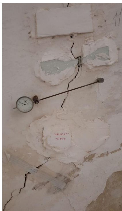
6-picture. A clock-Type Indicator was installed on the cracks that appeared on the wall of the large room
