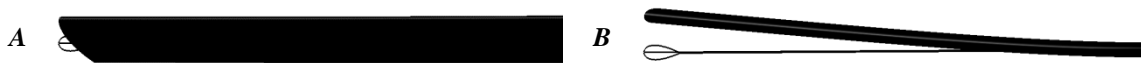
Figure 2. The deflection of the rotor blade of the helicopter from the initial position at eigenfrequencies of 0.17124 Hz (A) and 11.739 Hz (B).
