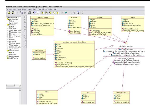
Pic. 2 - The class diagram (Class diagram) to select the type of special machines.
