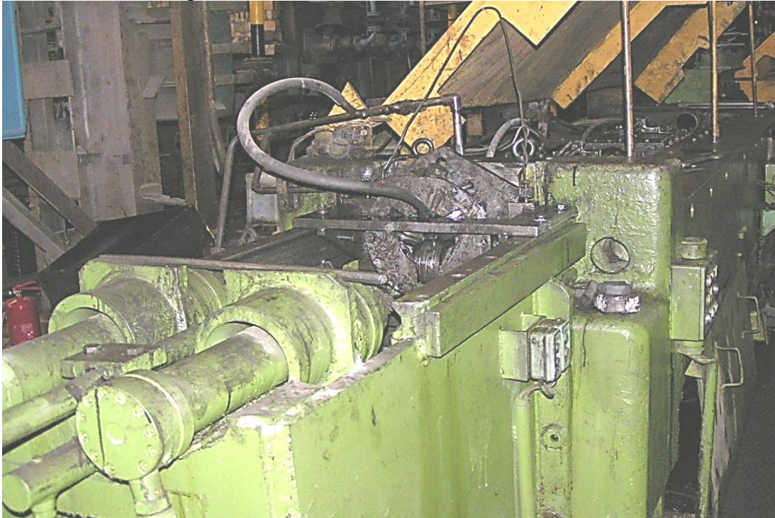
Figure 2 - Line for drawing and finishing bars with dual set of the housingless roller dies.
