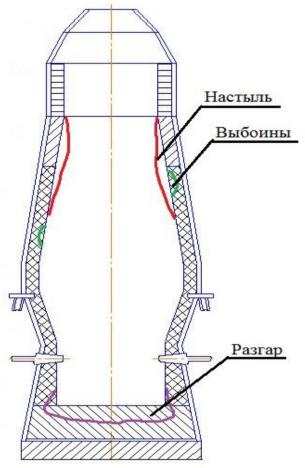
Figure 1 - Lines of the blast furnace.
