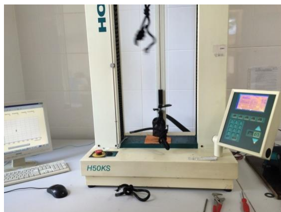
Figure 6 - Static test machine for tensile, compression, shear and bending materials, type H50K-S with interchangeable cells
