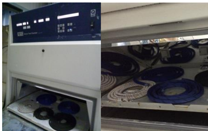
Figure 1- Aging equipment for determining exposure to artificial radiation (xenon) - Q-SUN xenon
