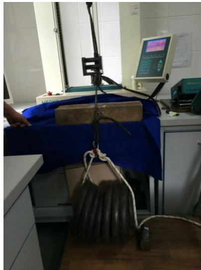
Figure 5 - Exposure to abrasive edges
