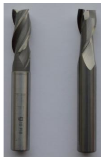
Figure 2 – The tools for milling: the high-speed end milling cutter with the diameter of 10 mm (left); the carbide end milling cutter with the diameter of 10 mm (right).
