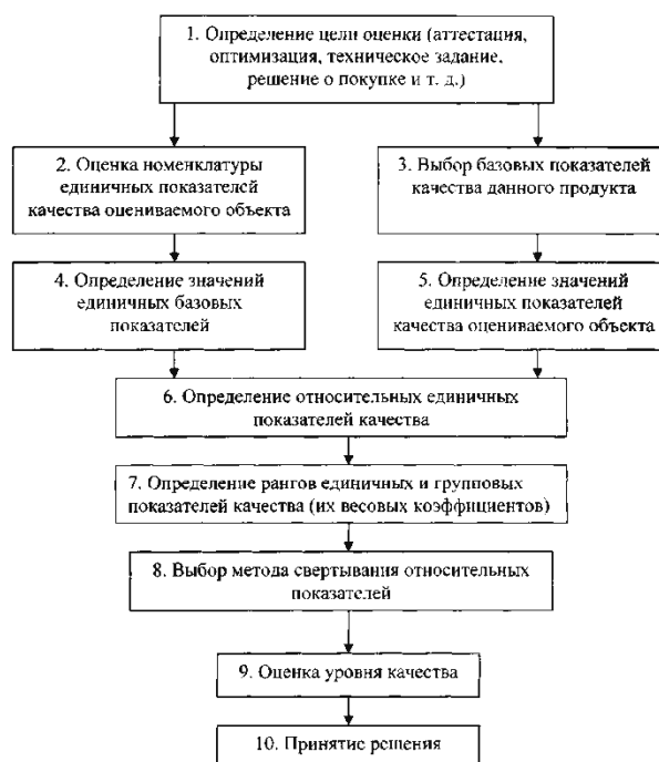
Figure 24 - Algorithm for a comprehensive assessment of the quality level of an object
