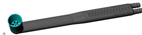
Fig. 6. The developed design of the removable nozzle for the hydro vacuum aspiration of the palatine tonsils lacunae
