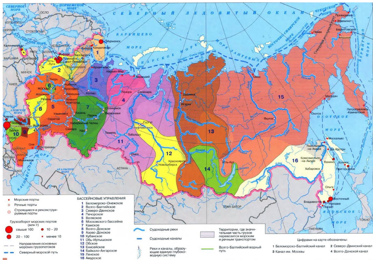
Figure 4. Characteristics of river transport routes of the Russian Federation and the regions of the Russian Arctic
