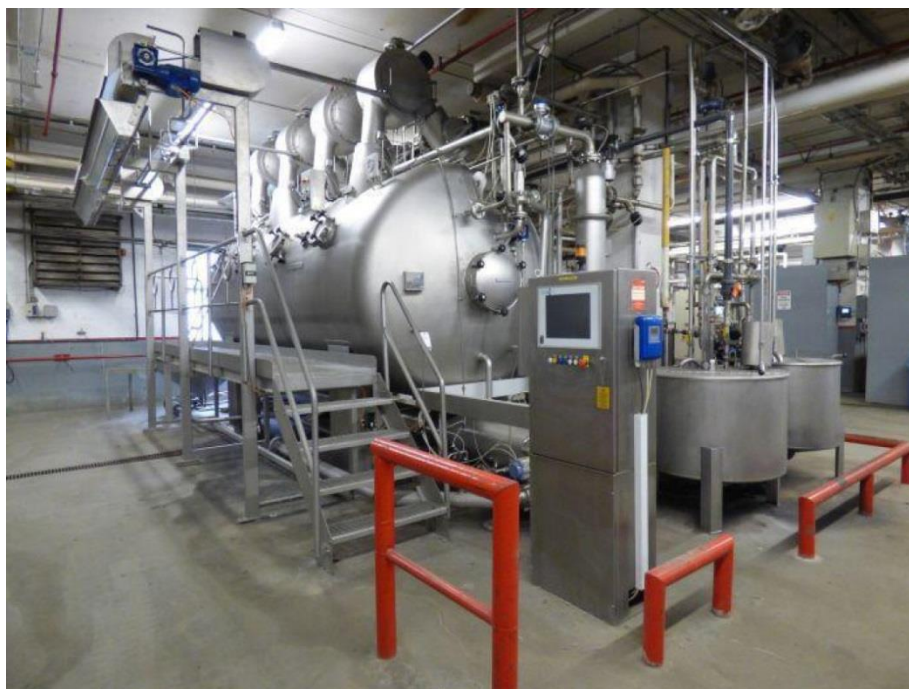
Figure 15. Luft-roto-plus ejector dyeing machines for the production of bleached, plain-dyed, printed fabric in a wide range of colors
