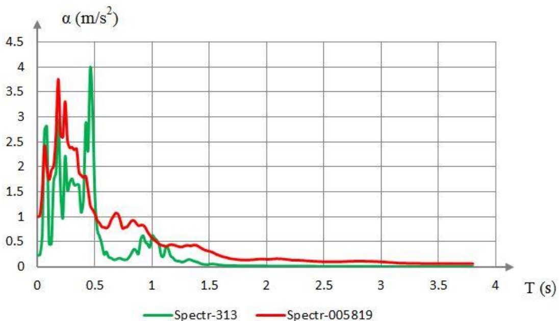
Fig. 7. The vertical normalized spectrum of the Kalamata earthquake (code: 005819) and the response spectrum of the superstructure with a scheme L=42.0+63.0+42.0 m
