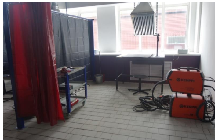
Figure 5. Welding station in the workshop.
