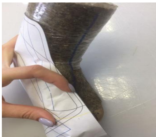
Figure 22. The position of gluing the primer model on the block
