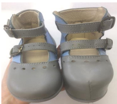
Figure 32. Shoe design with a seam on the vamp
