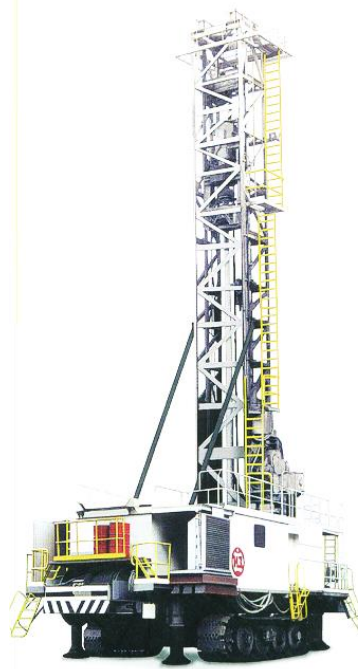
Figure 1. Quarry drilling rig 4SBSH - 200 - 40 with cartridge-type VPM.
