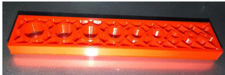
Figure 4. The partially printed part on the 3D printer.
