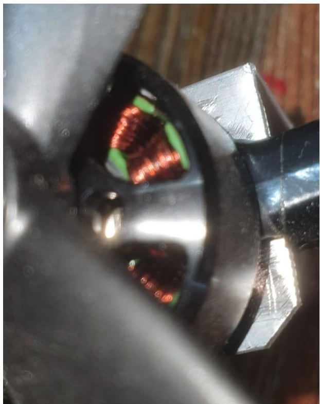
Picture 3. Overheating of the motors.
