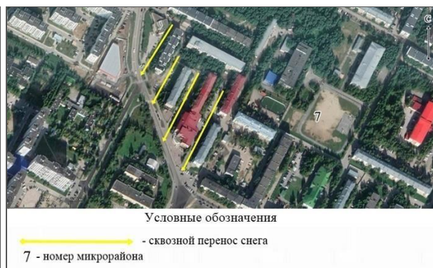
Figure 8. Layout of buildings in the microdistrict No. 7 of the city of Nizhnevartovsk, reducing snow drifts
