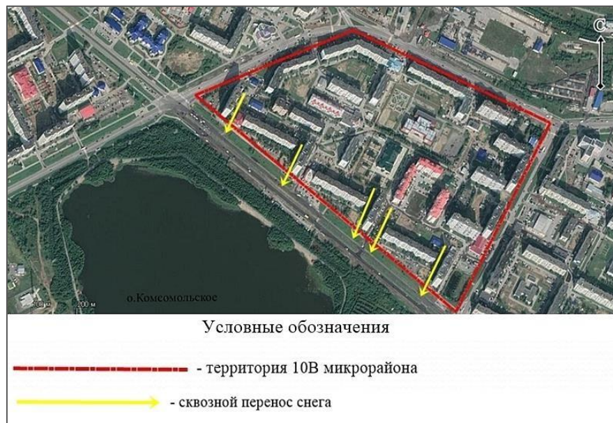
Figure 11. Layout of buildings in microdistrict No. 10B of the city of Nizhnevartovsk, reducing snow accumulation
